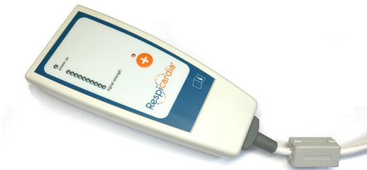
Figure 14 The remedē System Programmer Wand
